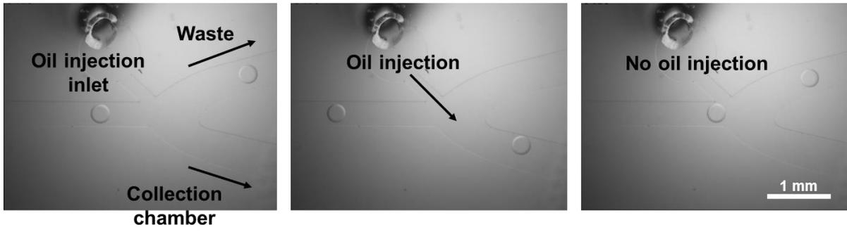
**Figure S6.** On-chip droplet sorting. Transient oil injection temporarily changes the flow direction of the droplets from the waste outlet to the collection chamber, allowing for a particular droplet to be selectively recovered.
