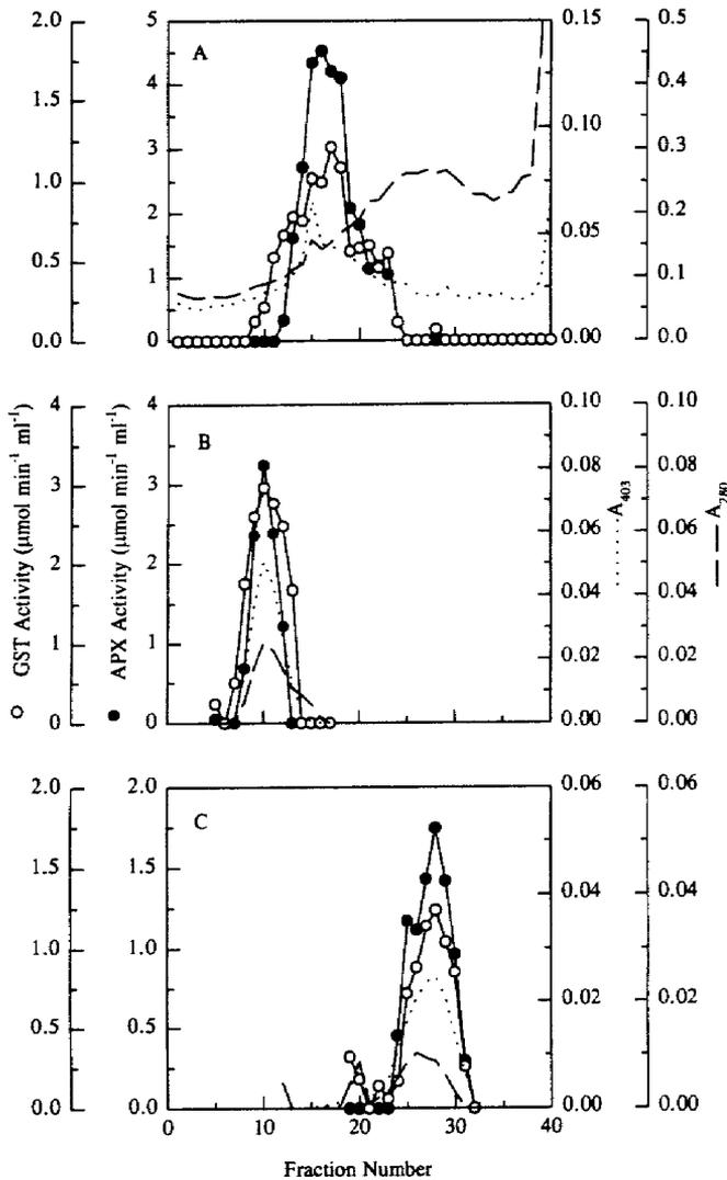
Fig. 2. Chromatographic purification of the GSH-conjugating and APX activities from corn shoots. Chromatography was performed on phenyl-Sepharose hydrophobic-interaction (A), Q-Sepharose FF anion-exchange (B), and Sephacryl S-200 gel filtration (C) columns. The GSH-conjugating activity with 4-CA was determined with the colorimetric assay.
